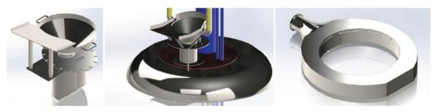
The manway nitrogen purge hopper serves as an engineering control to help maintain low oxygen concentrations within a process vessel during the manual addition of solids. This device utilizes a safe pneumatically opened flap valve that reduces the amount of time the tank is opened to the room environment. A full perimeter annular ring injects nitrogen at dual flow rates to dilute oxygen concentrations.
